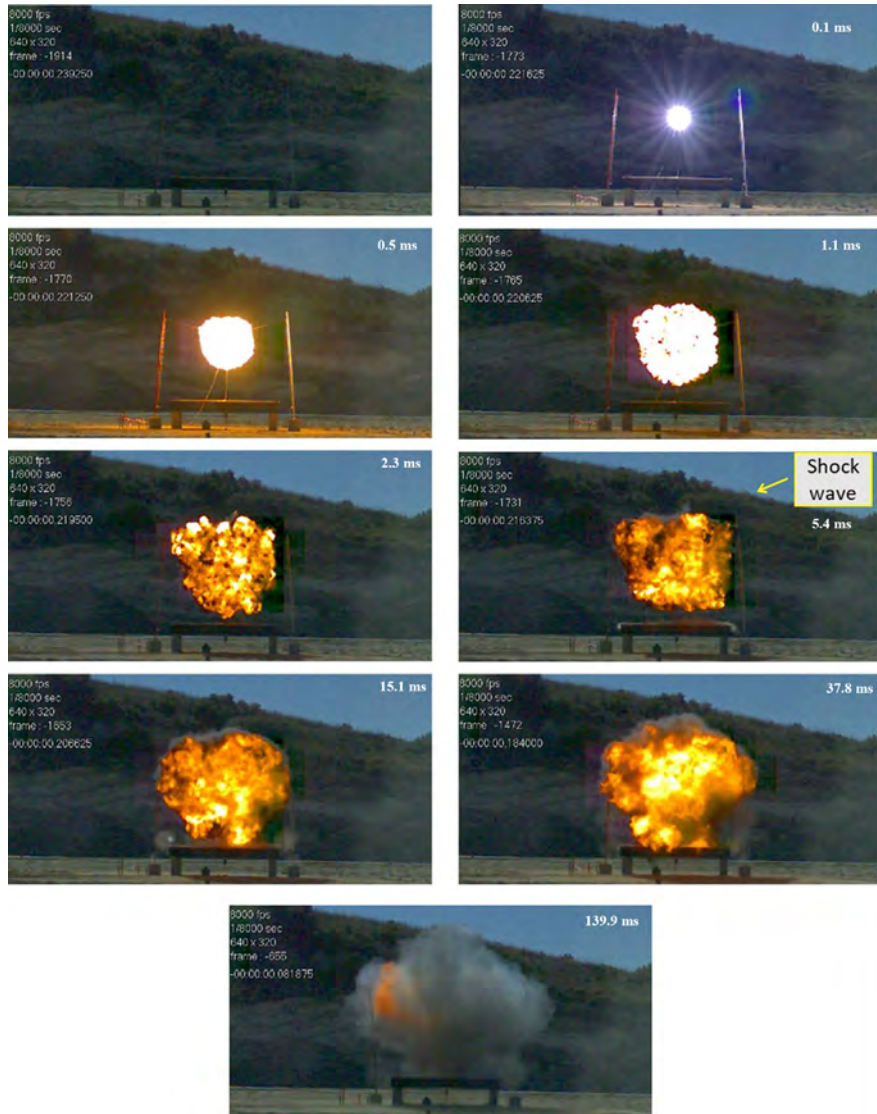
Figure 9. Sequence of images of test number 4 (3.2 kg TNT equivalent) taken with the high-speed camera.
