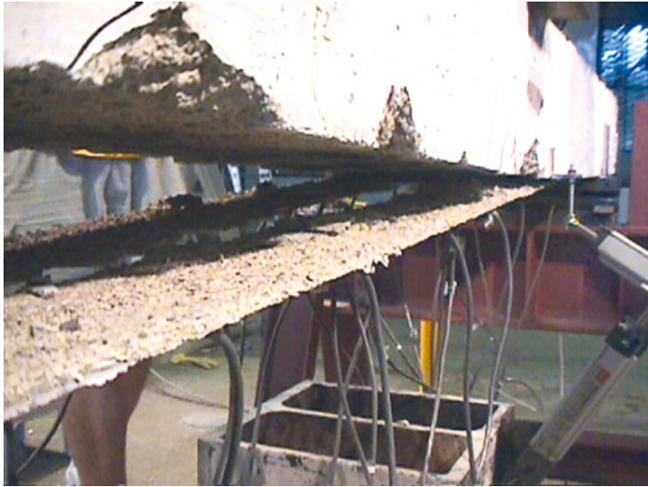
Figure 5. Debonding of the CFRP strengthening system [30].
