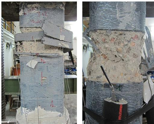
Figure 6. Failure mode of FRP confined concrete.
