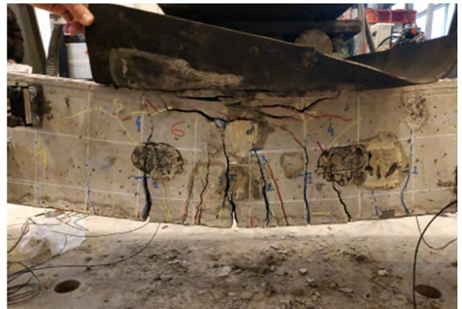
Figure 5. Crack pattern at failure of beam T3a.
