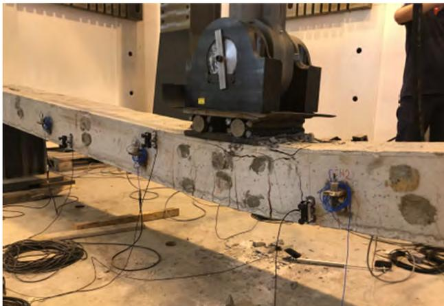
Figura 6. Crack pattern at failure of beam T4a.
