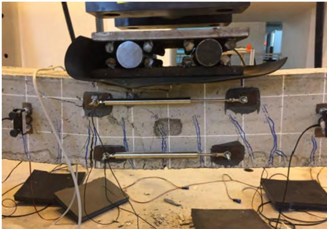
Figure 3. Crack pattern at failure of beam T1.
