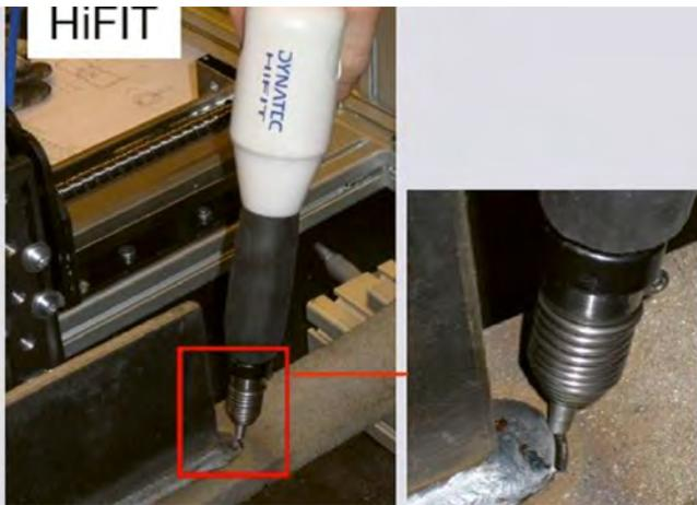
Figura 8. Tratamientos Post-soldadura High Frequency Impact Treatment (HiFIT).
