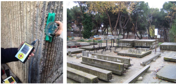
Figure 8. Left the corrosion rate meter in a column with rough finishing. Right: exposure site and the garden of the IETcc to study the effect of the climate into the corrosion of several concrete elements.
