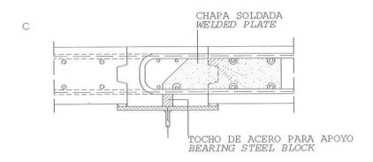
Figura 13. Junta entre paneles. Figure 13. Panel joints.
