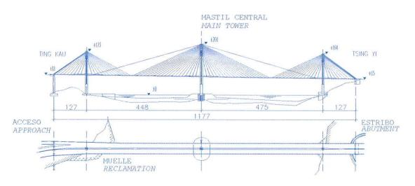
Figura 2. Alzado y planta con dimensiones principales. Figure 2. Elevation and plan with main dimensions.
