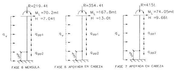
Donde  $q_v$ =0.0372t/m ,  $q_{pp1}$ =6.75t/m si h > 35m,  $q_{pp2}$ =12.375t/m si h > 35m,  $q_{pp1}$ =6.00t/m si h < 35m,  $q_{pp2}$ =12.000t/m si h < 35m,
