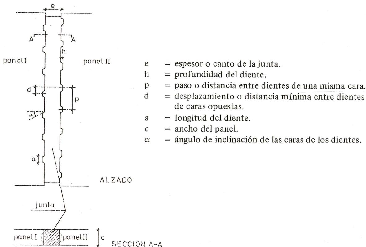
Fig. 2. Junta vertical.
