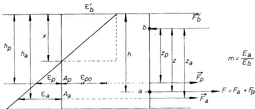
$$\omega_a = \frac{A_a}{bh_a} \quad \omega_p = \frac{A_p}{bh_a} \quad \bar{\omega}_a = \omega_a \cdot \frac{\sigma_{ak}}{\sigma_{bk}} \quad \bar{\omega}_p = \omega_p \cdot \frac{\sigma_{pk}}{\sigma_{bk}}$$
