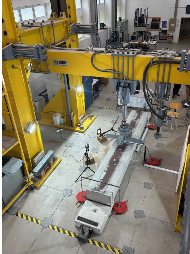
Figure 2: Beam being tested in hogging configuration.
