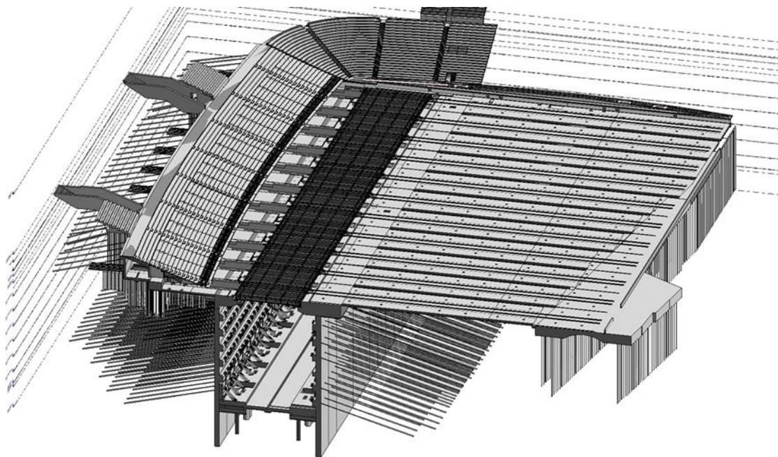
**IMAGEN 35 - LOSA DE CARRILES Y ANCLAJES PANTALLAS HIPOGEO**
