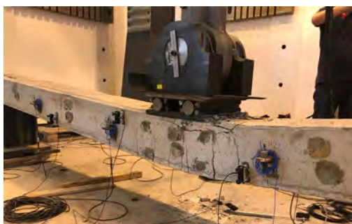
Figura 1. Crack pattern at failure of beam T4a.
