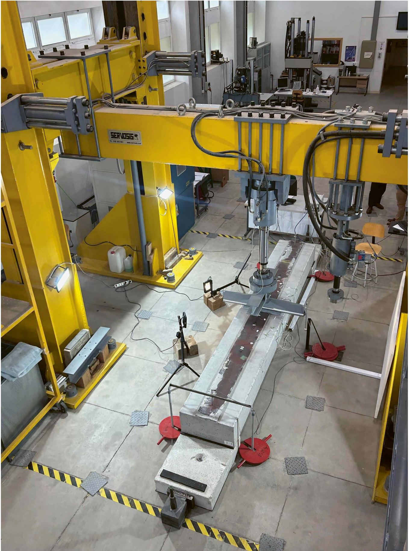
Figure 2: Beam being tested in hogging configuration.
