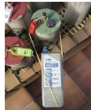
f) Probe measuring internal RH and T.
