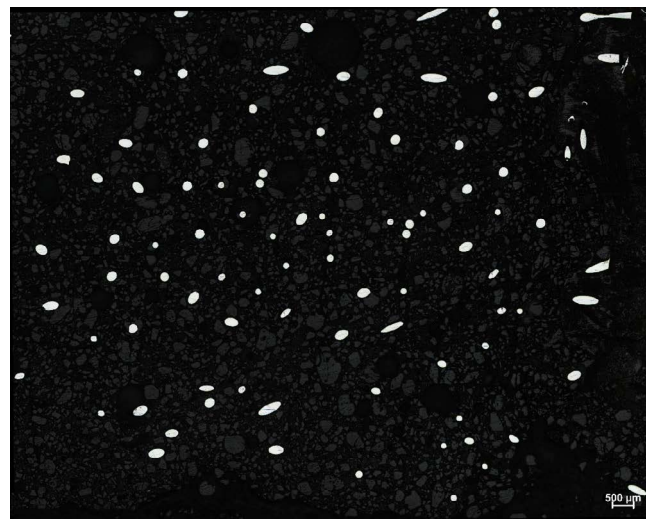
Figure 11. Image of Steel Fiber Orientation and Dispersion of F80/20_196 Mix.
